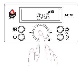
3. Turn the dial clockwise to select the high altitude setting for the application. (Default setting is '0-2' and high elevation is above 2,000ft as sea level.
