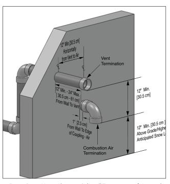
Fig. 7 - Direct Vent - Alternate Sidewall Termination of Vent and Combustion Air Piping
