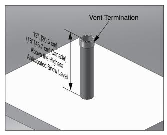
Fig. 14 - Category - IV - Vertical Termination of Vent Pipe
