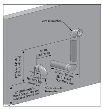
Fig. 6 - Direct Vent - Sidewall Termination of Vent and Combustion
