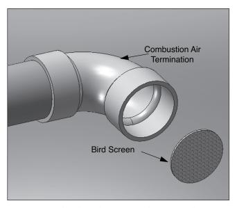
Fig. 10 - Sidewall Combustion Air Bird Screen Installation
