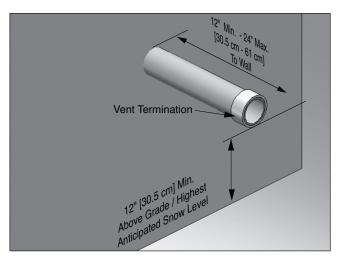
Fig. 17 - Category IV - Sidewall Termination of Vent Pipe
