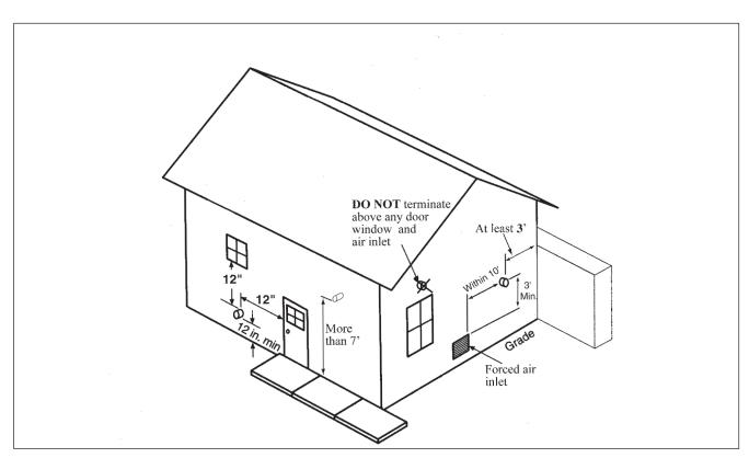
Fig. 2 - Termination Clearances of Direct Vent System
