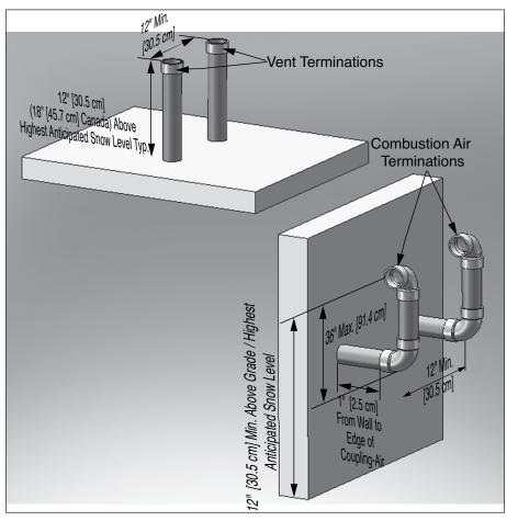
Fig. 13 - Direct Vent - Vertical Vent and Sidewall Combustion Air Terminations of Multiple Prestige Boilers
