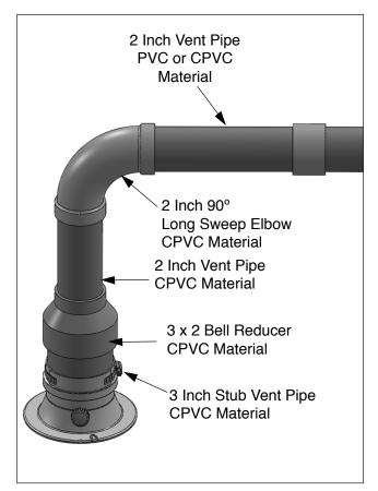
Fig. 21 - 2" CPVC/PVC Venting System Horizontal
